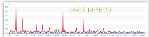
FFT Plots automatically generated by MultiViz Vibration indicating the most relevant timestamps in each operational mode
