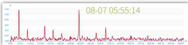
FFT Plots automatically generated by MultiViz Vibration indicating the most relevant timestamps in each operational mode
